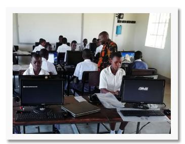
A thin client system consists of a cluster of GreenBridge Computing devices that are connected together by cables to a server to create a network. Each device is also connected to its own keyboard, mouse, and screen.
